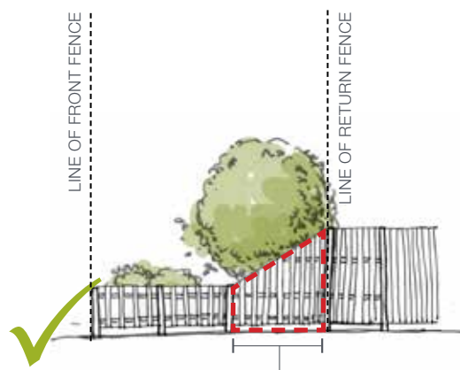
Transition height between 2 fence posts
