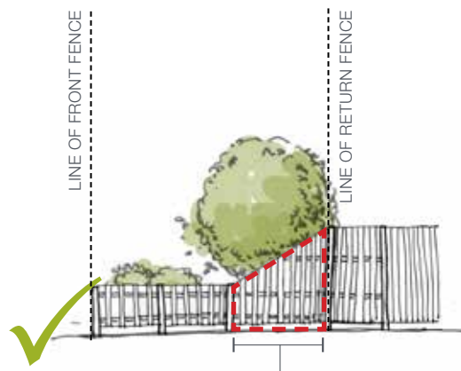
Transition height between 2 fence posts
