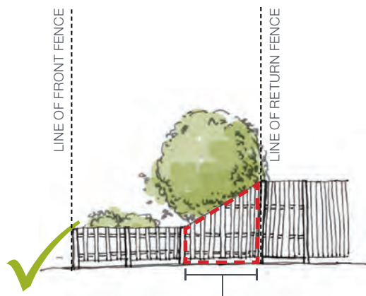
Transition height between 2 fence posts
